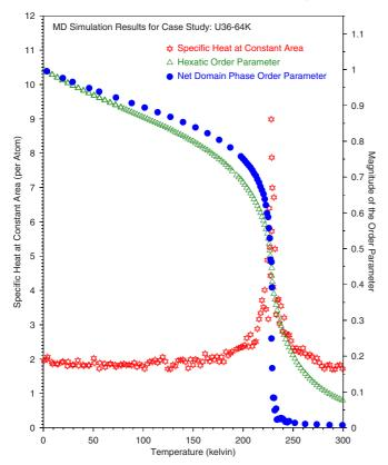
FIG. 1. (Color online) The hexatic order parameter, the NDP order parameter, and the specific heat for case study U36-64K of Xe/Pt, showing the alignment of the peak in the specific heat with the sharp drop in value of  $\psi_0$ . The density is  $\rho_p$ .
