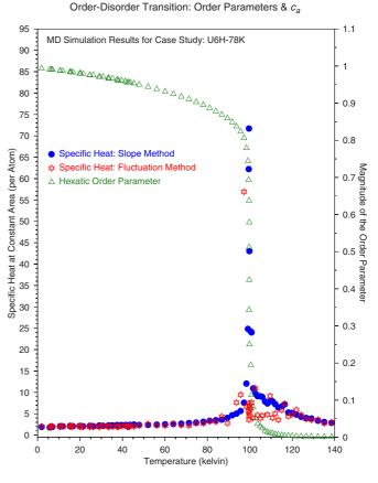
FIG. 2. (Color online) The hexatic order parameter and the specific heat for case study U6H-78K of Xe/Gr, comparing methods for the calculation of the specific heat. The average density is about  $\rho_g/2$ .
