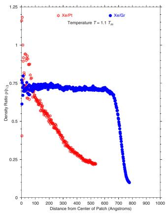
FIG. 3. (Color online) Comparison of the density profiles for patches of Xe/Gr (case study U6H-78K;  $T_m \simeq 100$  K;  $\rho \simeq \frac{1}{2}\rho_g$ ) and Xe/Pt (case study U36H-20K;  $T_m \simeq 150$  K;  $\rho \simeq \frac{1}{2}\rho_p$ ) just above the melting (order-disorder) transition.
